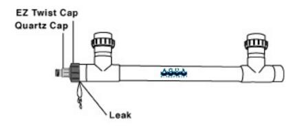
Untwist and check that the O-ring is seated in the top of the EZ-Twist cap. Hand-tighten until leak stops. Do not use a pipe wrench, pliers or any other tool. Hand-tighten only.
