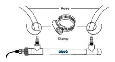
5. Do not install lamp(s) or electrical components yet. After all the connections have been made turn pump on and run it for five minutes to check for leaks.
