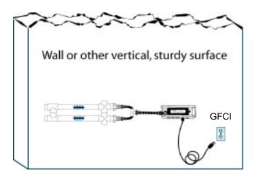
3. Plug the lamp(s) into the lamp end connector(s) located at the end of the wiring harness. Make sure the lamp(s) is plugged in all the way and flush with the lamp end connector(s). Insert the lamp into the quartz sleeve.
