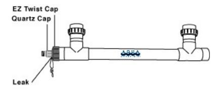
Undo quartz cap and push rubber seal into the housing evenly. The rubber seal should be 1/2 in and 1/2 out. Redo quartz cap and finger tighten. Do not use a pipe wrench, pliers or any other tool. Hand-tighten only.
