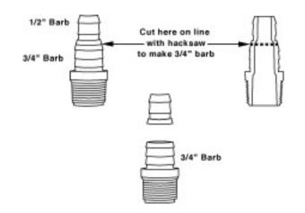
b. The barbs have been Teflon taped for you to prevent leakage. Install barbs, hose and hose clamps.
