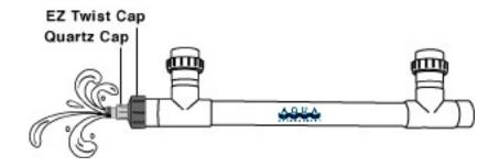
The quartz sleeve is broken and needs to be replaced. A broken quartz sleeve is not, nor is any damage caused as a result of a broken quartz sleeve, covered under warranty. Contact your dealer for a replacement. (See INSTALLING A REPLACEMENT QUARTZ SLEEVE on page 17).
